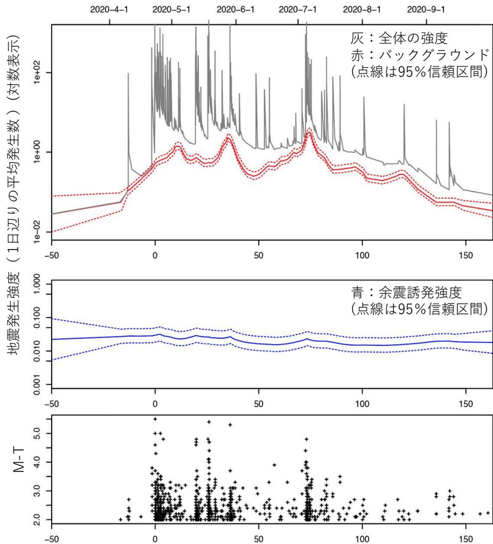
非定常ETAS:  $\lambda_{\theta}(t|H_t) = \mu(t) + \sum_{\{i:S \leq t_i < t\}} K_0(t) e^{\alpha(M_i - M_c)} / (t - t_i + c)^p$
