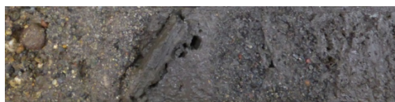
★1; 2.35-60 m; Alternation of sandy mud and sand layers
